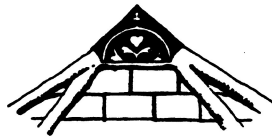
Mediaeval tile fragment used as ridge tile closer over porch
